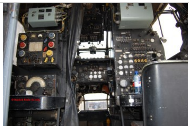
T1154/R1155 installation in a Shackleton
