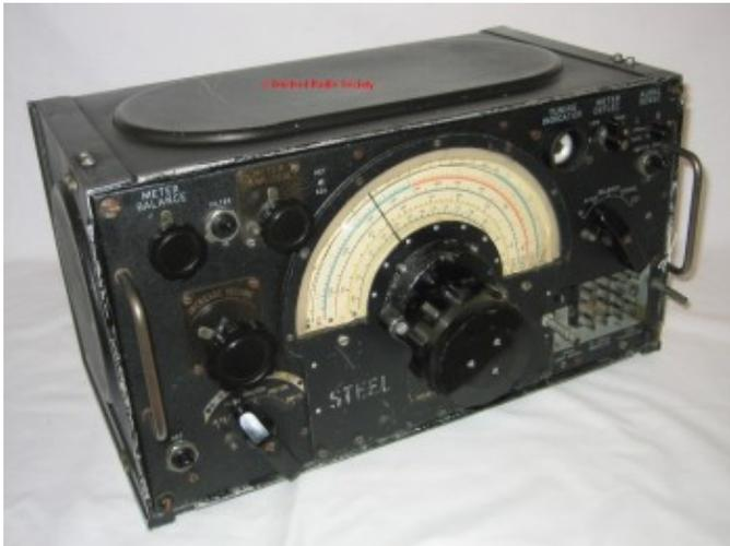
For reception of communications signals, the receiver could be connected to either fixed wire aerials mounted on the aircraft or long trailing line aerials. A fixed aerial was normally used for the HF ranges, and the trailing aerial on the medium frequency (MF) ranges. The DF aerial, such as an Air Ministry Type 3 or 4 Loop, was the standard fit for the direction-finding facility.
