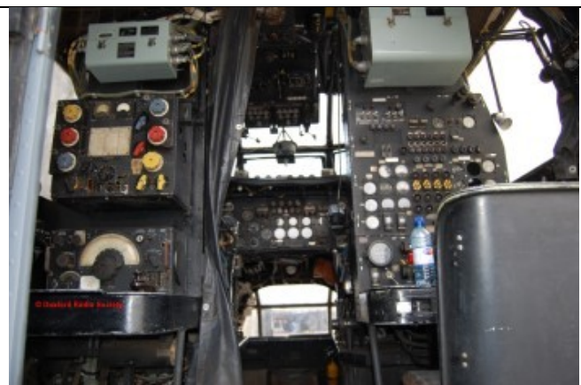
T1154/R1155 installation in a Shackleton
